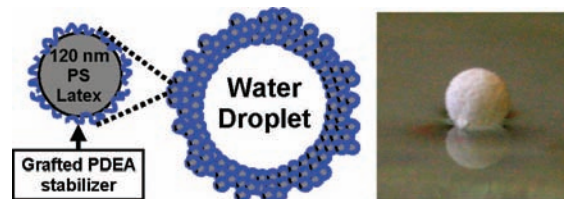
Figure 1. Schematic representation of a typical millimeter-sized “liquid marble” coated with latex multilayers. A digital image of such a “liquid marble” placed at the air/water interface is also shown.
